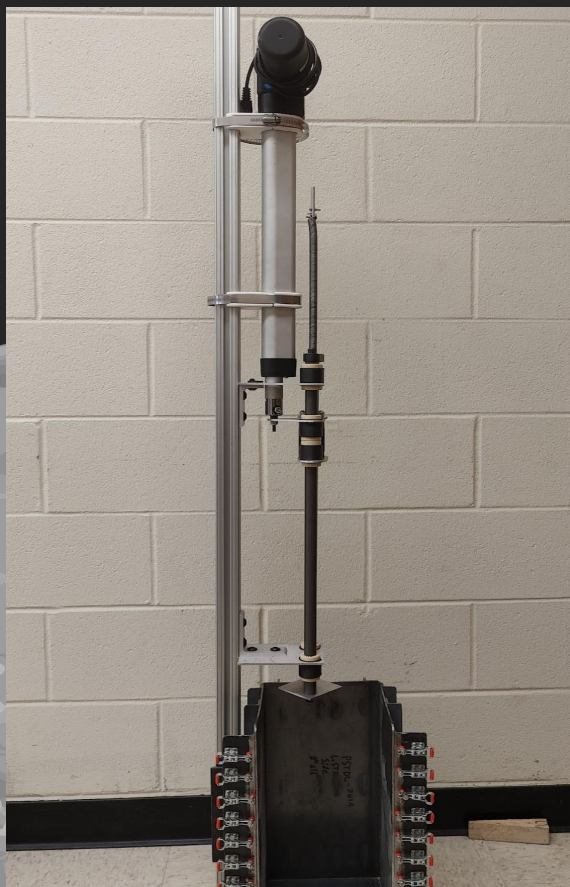
Figure 1: Single Pin Test Set-up
